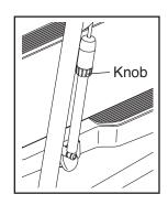
**more you weigh, the firmer the shock cylinders should be.** When running on the treadmill, set the firmness level to at least 16. If the shock cylinders make a knocking noise as you run on the treadmill, increase the firmness level.
